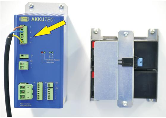
Connect the AKKUTEC to the mains (230VAC)
