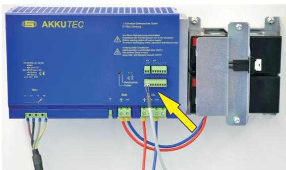
Wiring of the temperature sensor
